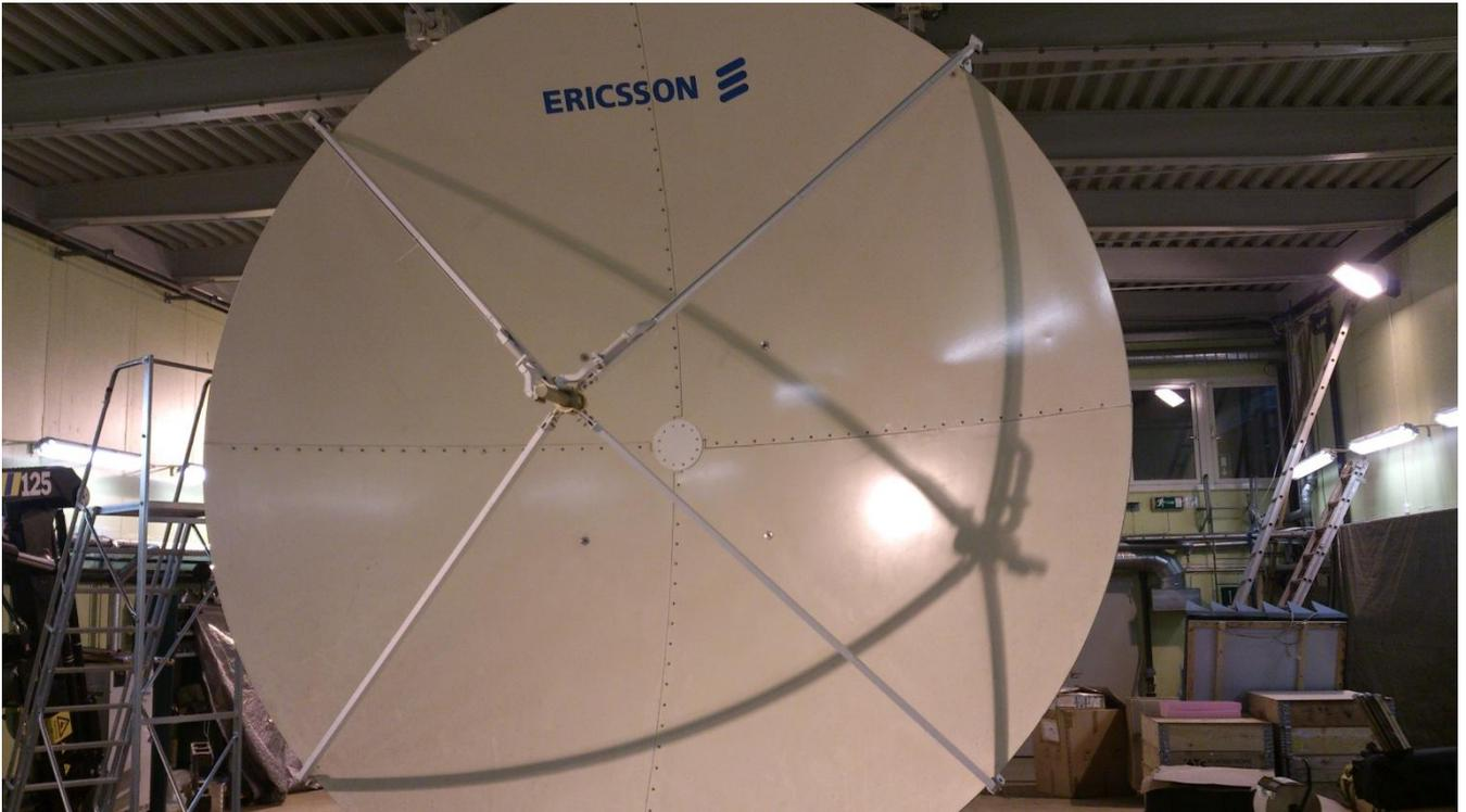
The antenna fulfil very demanding requirements concerning low side lobes, high antenna gain, similar antenna gain in H and V and very good cross polarization isolation
